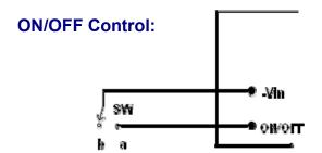
The converter output can be disabled by moving SW to position "a" – connected to –Vin with voltage level between -0.7 and 0.4V.
