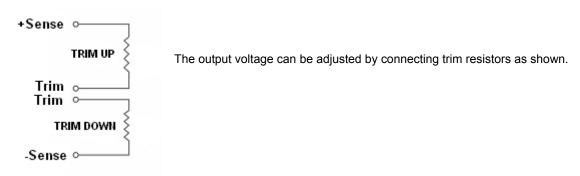
The values can be determined according to the following formulas where  $\Delta$ % is the desirable voltage adjustment in percentage and Vo is the Nominal value of the Output Voltage:
